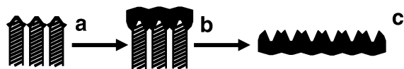
Figure 3. Preparation process of ordered nanoring arrays: (a) beginning of metal deposition on AAO film; (b) thicker metal film was deposited; (c) metal film with ordered arrays of nanorings after removing AAO film.
